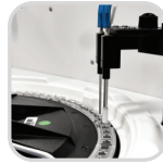
Probe Mixer Berbahan Politetrafluoroetilena Anti Residu
